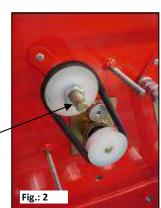
3. Fix the supplied indicator to the agitator shaft (M10 threading) (with 2x 17mm wrenches).
